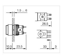
A = Solder terminal B = Plug-in terminal 2.8 mm x 0.5 mm C = Universal terminal 2.0 mm x 0.5 mm
