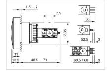
$B = Plug-in terminal 2.8 \times 0.5 mm$
