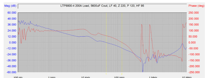
Figure 3. Measured Bode Plot of the LTP8800-4A
