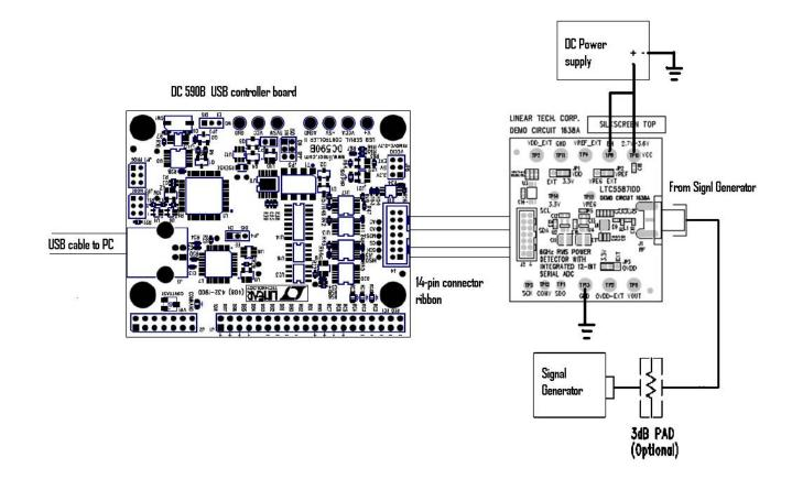
Figure 2. Proper test setup to connect DC1638A demo board to DC590A
