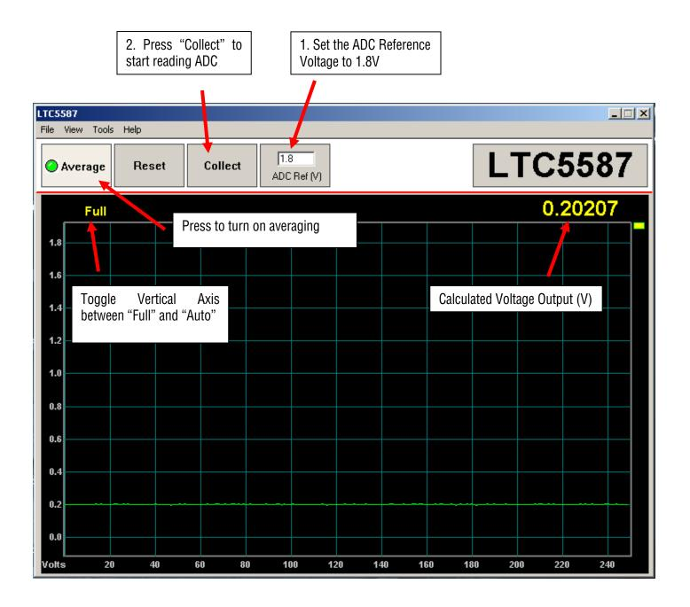
Figure 3. Front Control Panel for LTC5587. With no RF input signal.
