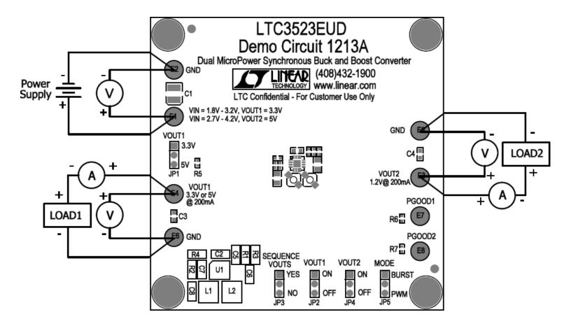
Figure 1. Proper Measurement Equipment Setup
