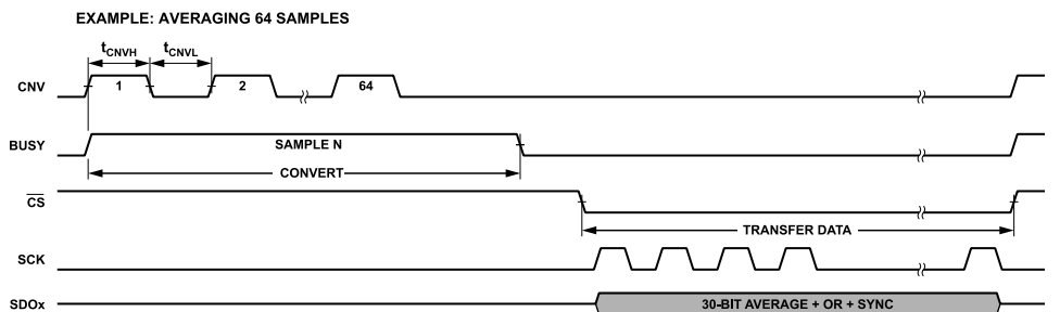
Figure 54. Example Conversion Cycle for Averaging Mode
