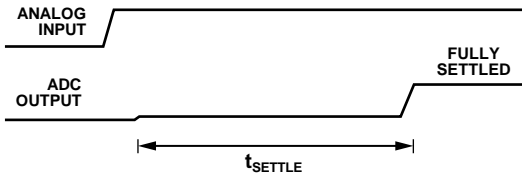
Figure 33. Step Input with Single Cycle Settling
