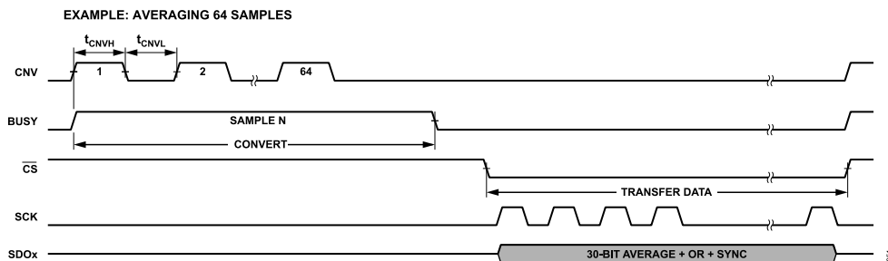
Figure 63. Example Conversion Cycle for Averaging Mode
