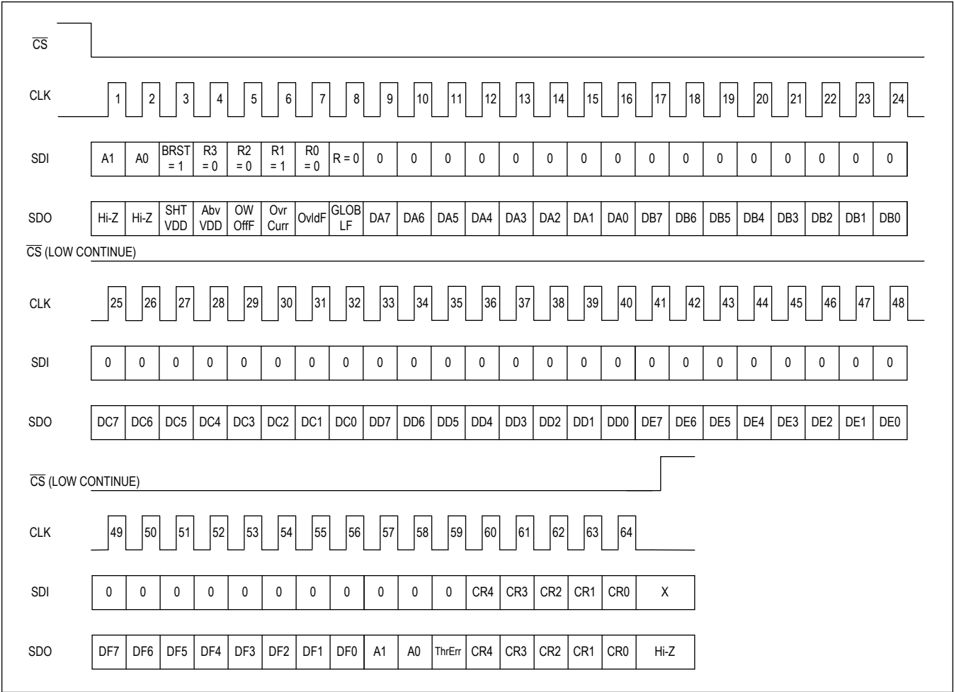
Figure 15. SPI Burst Read with CRC Enabled
