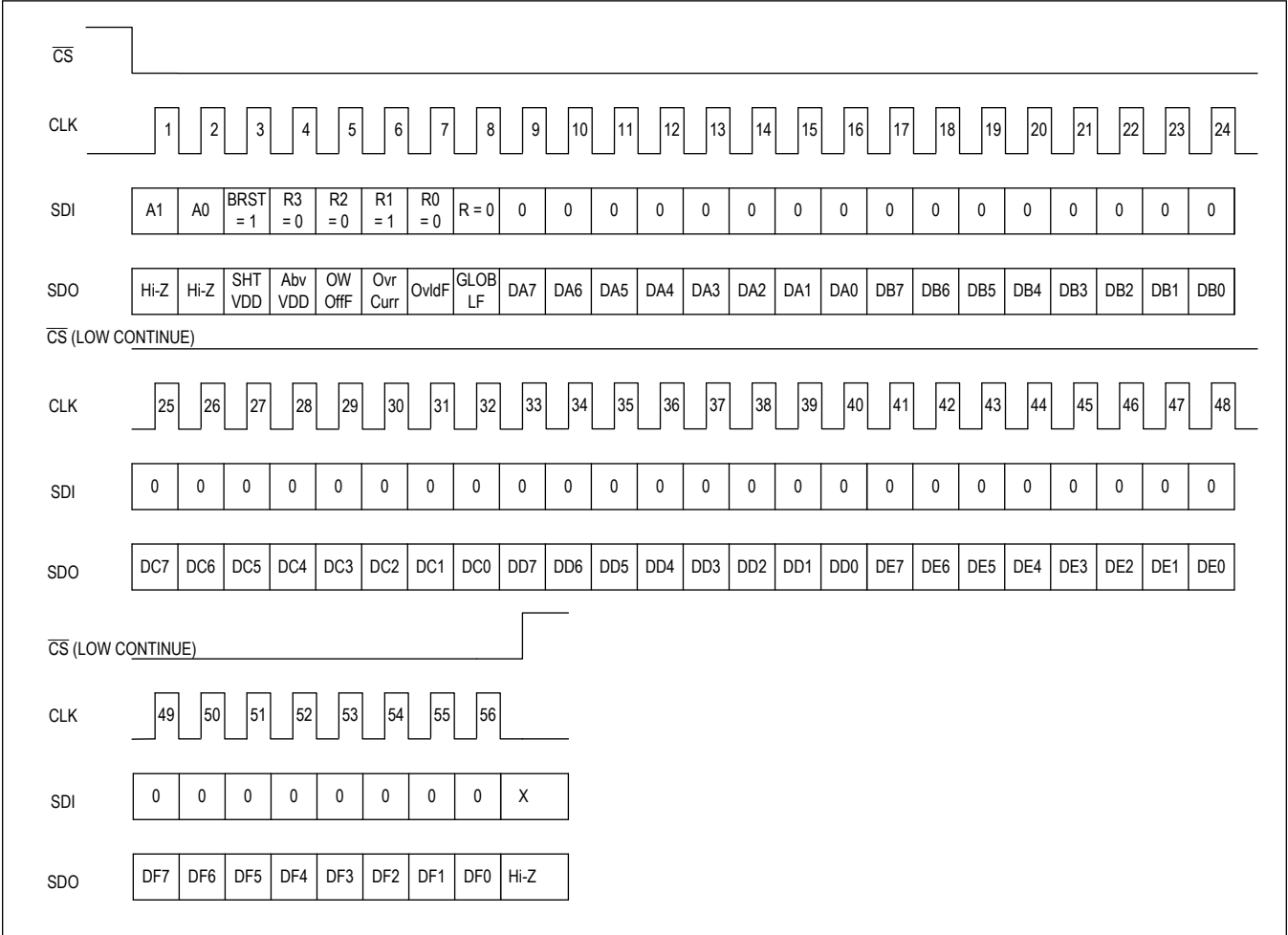
Figure 14. SPI Burst Read without CRC Enabled
