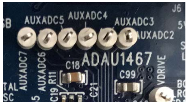
Figure 70. Auxiliary ADC Test Points Communications Header
