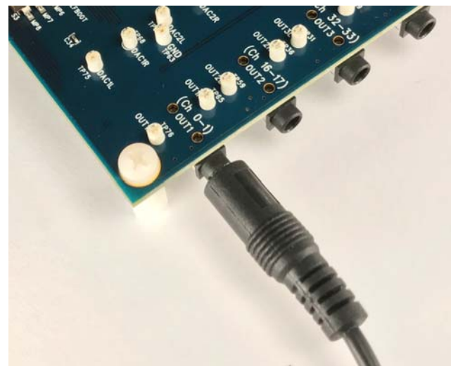
Figure 12. Analog Stereo Output Connection
