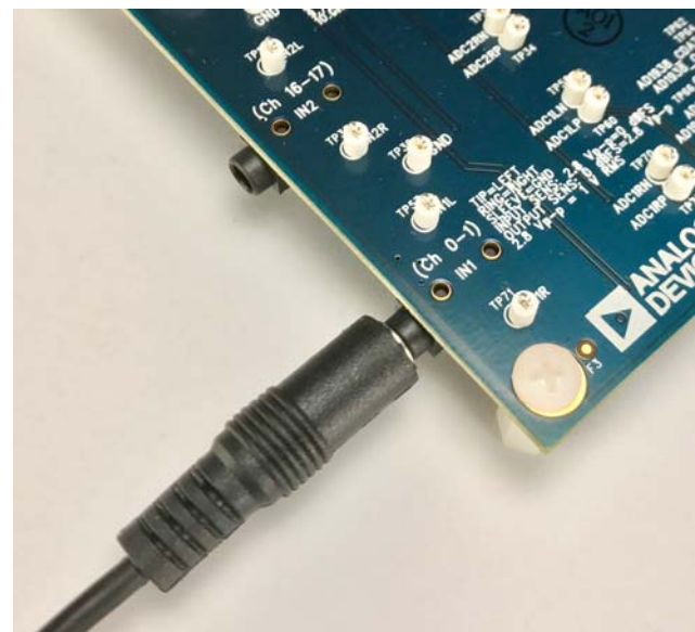
Figure 11. Analog Stereo Input Source Connection
