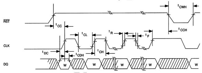
3-WIRE READ DATA TIMING DIAGRAM Figure 20
