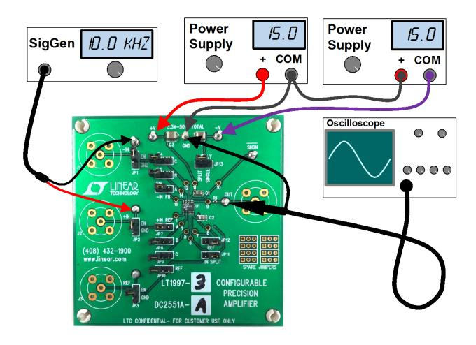
Figure 1. Proper Evaluation Equipment Setup
