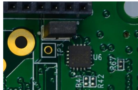
Figure 7. PC Temperature Circuit
