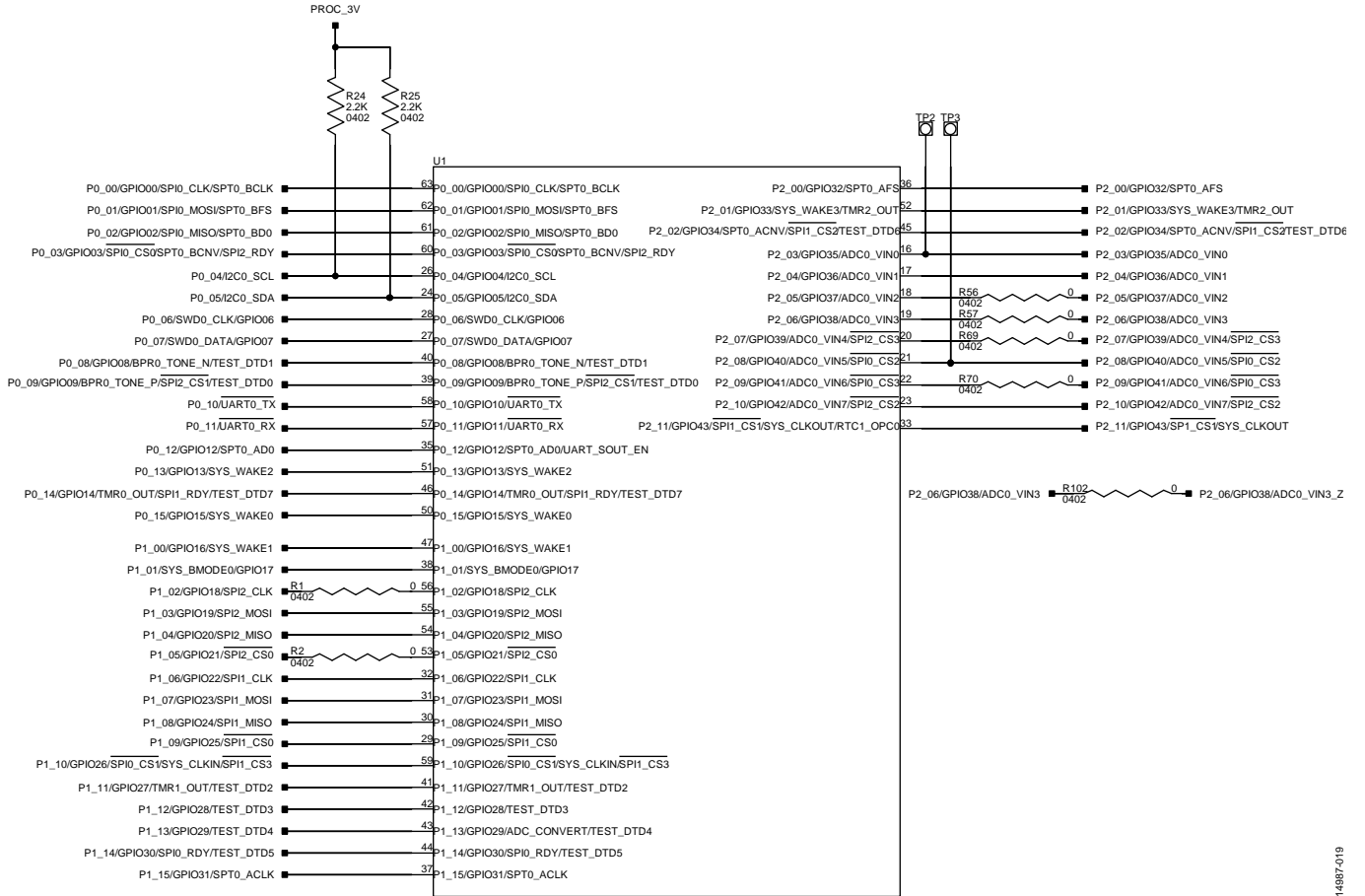
Figure 20. ADuCM3027/ADuCM3029 Microcontroller GPIO Schematic
