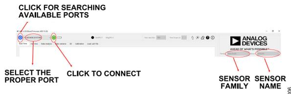
Figure 6. Hardware Detection
