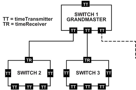
Figure 61. Time Synchronization Example for External Port Config
