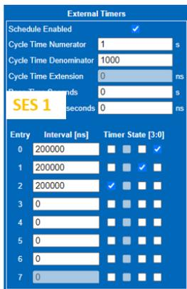
*Figure 92. Configured Schedule for Switch 1 Timers*
