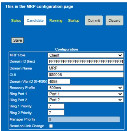
Figure 126. MRP Candidate Page: Switch 2, MRP Enabled as MRC (Client)
