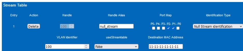
Figure 155. Talker Stream Configuration Example
