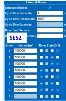
*Figure 93. Configured Schedule for Switch 2 Timers*
