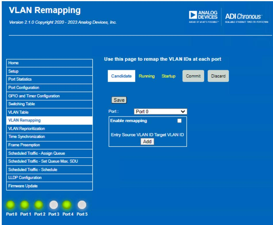
Figure 43. VLAN Remapping Page – Candidate View
