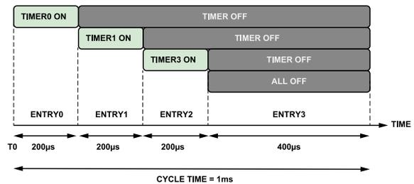
*Figure 94. Schedule for Switch 1 Timer Pins*
