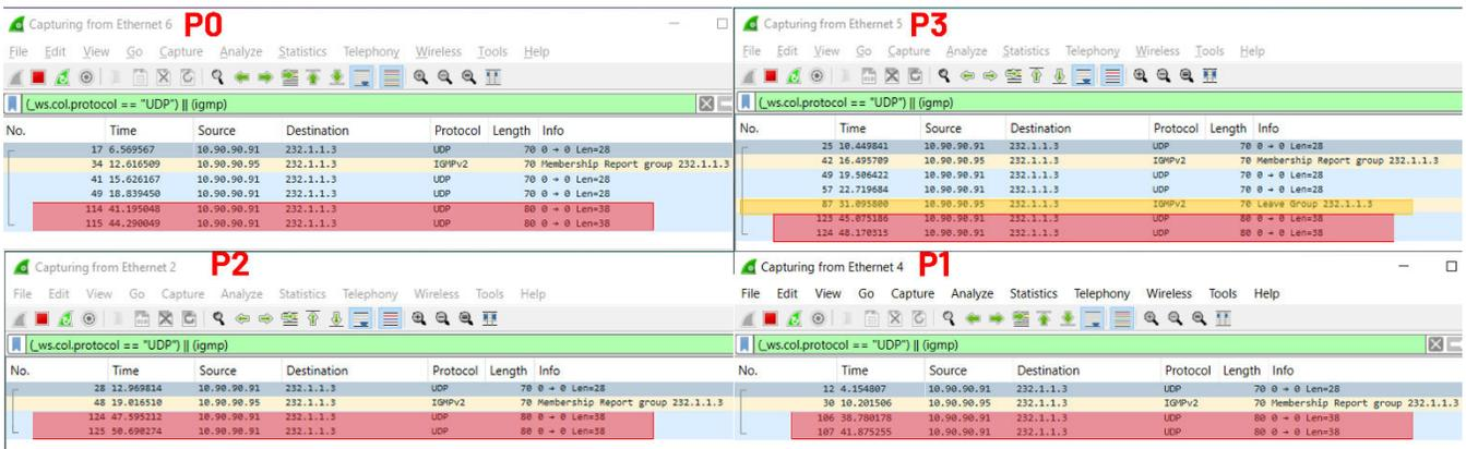
Figure 164. IGMPv2 – Leaving Message Scenario on Port P3
