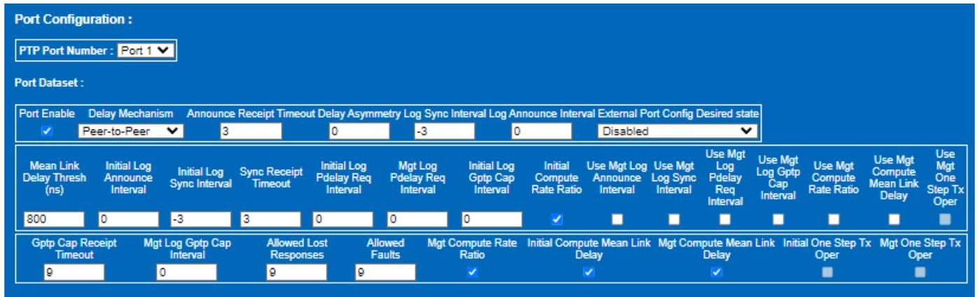
Figure 53. Time Synchronization Candidate Page – Port Configuration
