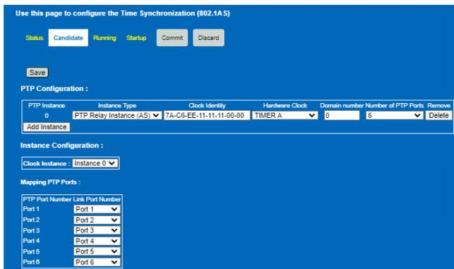
Figure 50. Time Synchronization Candidate Page – PTP Configuration
