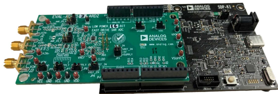
Figure 2. EVAL-AD4052-ARDZ and SDP-K1 Connections
