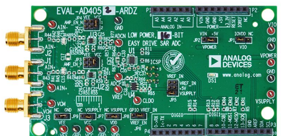
Figure 1. EVAL-AD4052-ARDZ Evaluation Board Photograph
