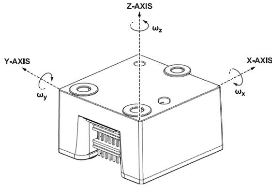
Figure 60. Gyroscope Axis and Polarity Assignments
