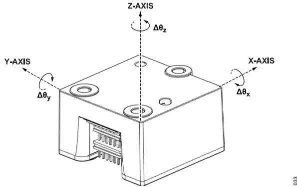
Figure 64. Delta Angle Axis and Polarity Assignments
