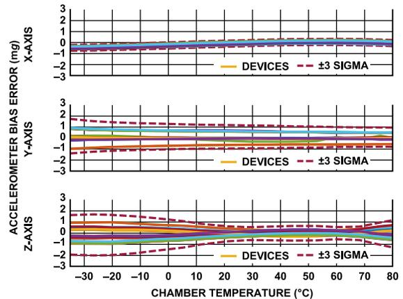
Figure 24. Accelerometer Bias Error vs. Chamber Temperature, ADIS16575
