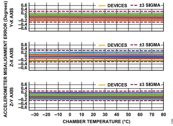
Figure 35. Accelerometer Misalignment Error vs. Chamber Temperature, ADIS16577
