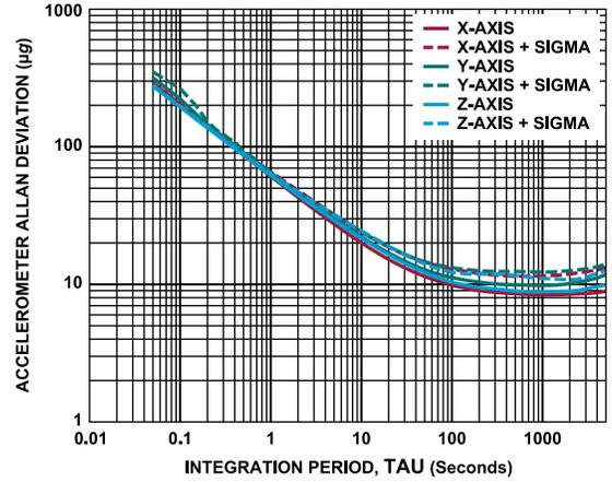
Figure 22. Accelerometer Allan Deviation,  $T_C = 25^\circ\text{C}$ , ADIS16576
