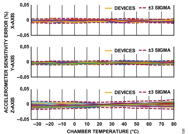
Figure 29. Accelerometer Sensitivity Error vs. Chamber Temperature, ADIS16577
