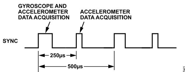
Figure 72. Sync Output Signal, Register MSC\_CTRL, Bits[3:2] = 11
