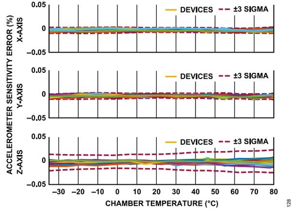
Figure 28. Accelerometer Sensitivity Error vs. Chamber Temperature, ADIS16576
