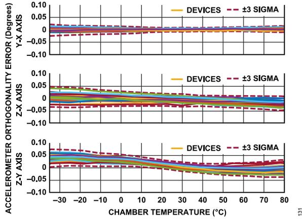
Figure 31. Accelerometer Orthogonality Error vs. Chamber Temperature, ADIS16576
