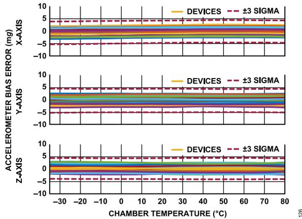
Figure 26. Accelerometer Bias Error vs. Chamber Temperature, ADIS16577
