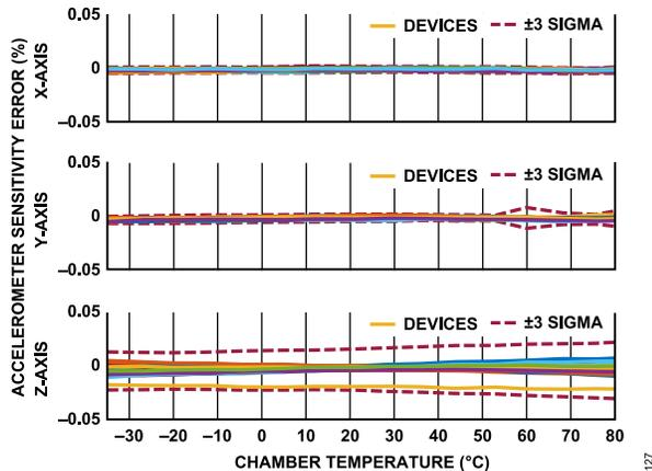
Figure 27. Accelerometer Sensitivity Error vs. Chamber Temperature, ADIS16575
