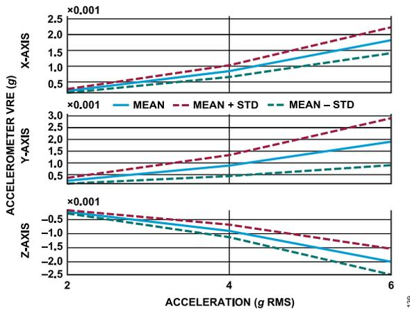
Figure 39. Accelerometer Vibration Rectification Error,  $T_C = 25^\circ\text{C}$ , ADIS16576
