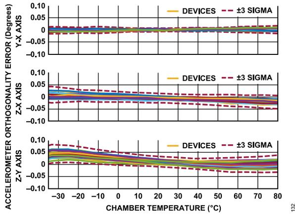
Figure 32. Accelerometer Orthogonality Error vs. Chamber Temperature, ADIS16577
