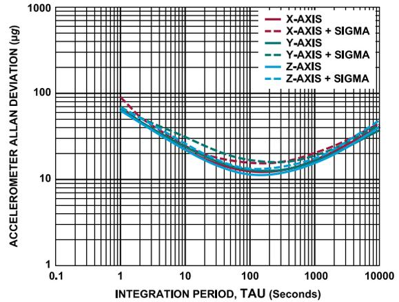
Figure 23. Accelerometer Allan Deviation,  $T_C = 25^\circ\text{C}$ , ADIS16577
