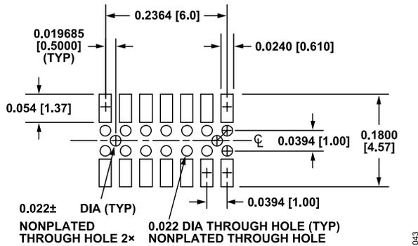
Figure 74. Mating Connector Design Detail
