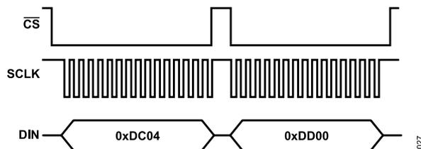
Figure 58. SPI Sequence for Writing 0x0004 to `FILT_CTRL`
