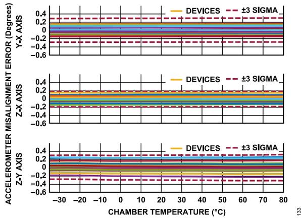
Figure 33. Accelerometer Misalignment Error vs. Chamber Temperature, ADIS16575
