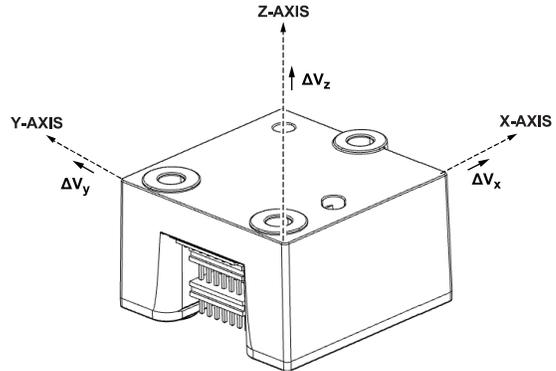
Figure 66. Delta Velocity Axis and Polarity Assignments
