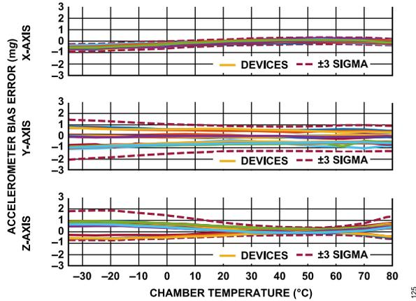
Figure 25. Accelerometer Bias Error vs. Chamber Temperature, ADIS16576
