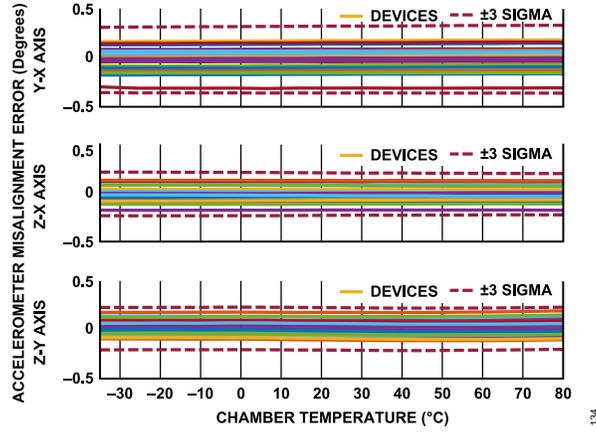
Figure 34. Accelerometer Misalignment Error vs. Channel Temperature, ADIS16576
