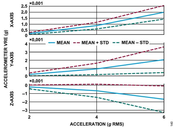
Figure 40. Accelerometer Vibration Rectification Error,  $T_C = 25^\circ\text{C}$ , ADIS16577
