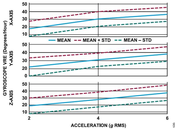
Figure 20. Gyroscope VRE,  $T_C = 25^\circ\text{C}$ , ADIS16576-3 and ADIS16577-3
