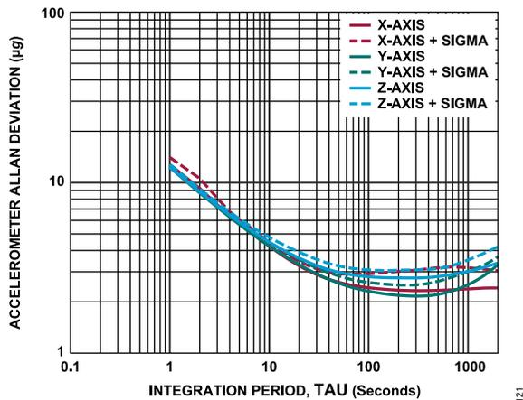
Figure 21. Accelerometer Allan Deviation,  $T_C = 25^\circ\text{C}$ , ADIS16575
