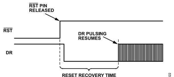
Figure 51. Data Ready Response During Reset ( $\overline{RST} = 0$ ) Recovery
