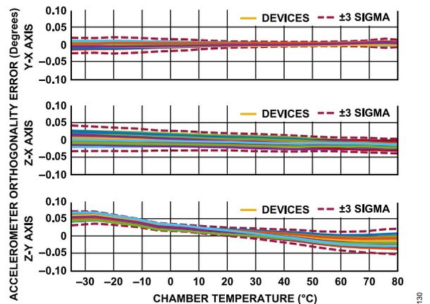
Figure 30. Accelerometer Orthogonality Error vs. Chamber Temperature, ADIS16575
