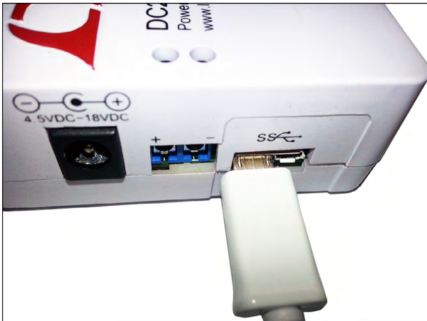
Figure 11. DC2086A USB Input Connector
