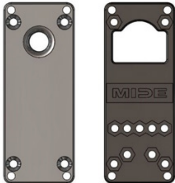
Figure 69: PPA-5008 clamp enclosure base and PPA-5009 clamp enclosure top are shown above. This base provides interfaces to clamp the piezo products, incorporate the wiring strain relief, utilize mounting magnets, bolt the base down to another structure, and secure the top, the mirrored base or even a PCB to the top.
