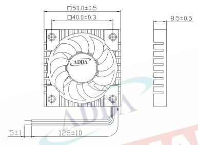
LEAD WIRES: UL 1571, AWG28, L = 125 +/- 10 mm Red = positive; Black = negative.
