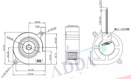
LEAD WIRES: UL 1571, AWG28, L = 130 +/- 10 mm Red = positive; Black = negative. White = FG
