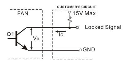
\*Transistor Q1 at "ON" position Collector current.....I<sub>c</sub>=10mA Max Saturation Voltage.....V<sub>oL</sub>=1.0V Max (Between Collector and Emitter at I<sub>c</sub>=10mA) \*Transistor Q1 at "OFF" position Release Voltage.....V<sub>OH</sub>=15V Max
