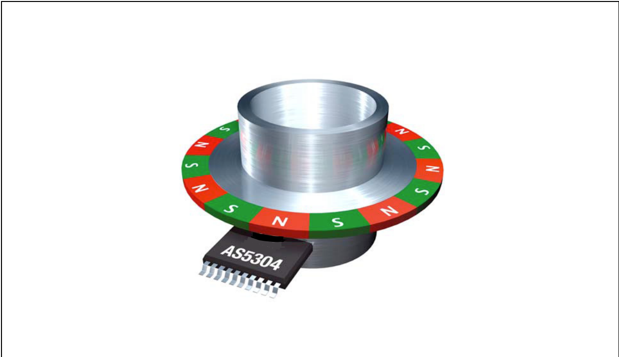
Figure 20: AS5304 (AS5306) with Multi-Pole Ring Magnet
