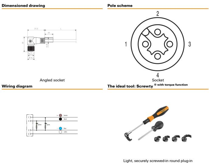
connectors. Screwty set DM / VPE: 1 / Order No.: 1920000000 Adapters: M12, M12 F, M8, M8 F
