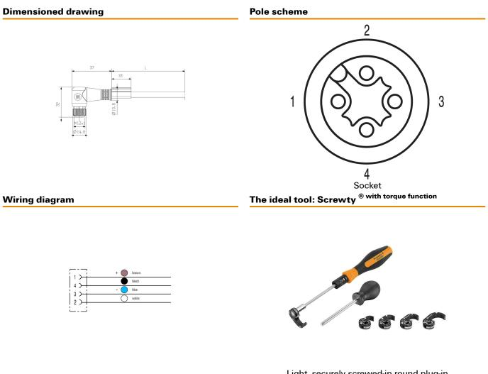
Light, securely screwed-in round plug-in connectors. Screwty set DM / VPE: 1 / Order No.: 192000000 Adapters: M12, M12 F, M8, M8 F
