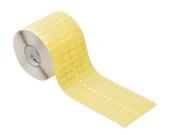
THM GEW woven-fabric labels are made from a very flexible cotton fabric. Delivery on reels for use with thermal transfer printers enables an adhesive layer which is thicker than that of A4 sheets for office laser printers. Together, this flexibility and the thick adhesive layer ensure higher adhesive strength and enable use on angular or round objects such as e.g. cables or hoses.
