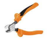
Cutting tools for conductors up to 8 mm, 12 mm, 14 mm and 22 mm outside diameter. The special blade geometry allows pinch-free cutting of copper and aluminium conductors with minimum physical effort. The cutting tools also come with VDE and GS-tested protective insulation up to 1,000 V in accordance with EN/IEC 60900.
