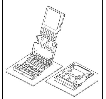
This is micro SD card cnnector of flip cover type that can approach from above the PC board surface.
