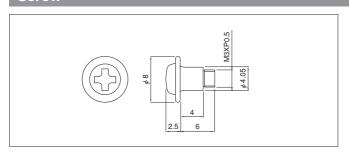
Note: Two screws are supplied for one receptacle housing, RPJ-26RS.
