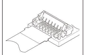
The FXV connector is a market require space saving and low profile 0.3mm pitch connector, and designed for corresponding to FPC with protrusions. As FPC with protrusions is used for this FXV connector, easy insertion operation, protection of incomplete insertion and miss-insertion are realized.
