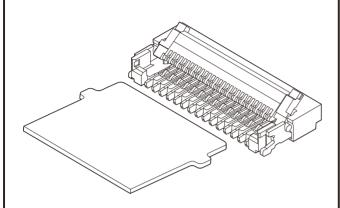
0.2mm pitch FVX connector for FPC has been developed for small portable equipment for which low profile and miniaturization are required. By using FPC with protrusions, the positioning accuracy of FPC is improved.
