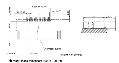
Note: 1. The PC board layout figure shown is viewed from the connector mounting surface.
