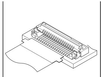
This connector features a mounting height of 1.3 mm and a FPC thickness of 0.3 mm with contacts located on the bottom. Moreover, it is designed to improve connection reliability by preventing incomplete mating and incorrect insertion of FPCs with protrusions.
