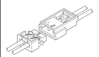
This is the wire-to-wire connector for DC power supply.
