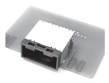
This HIE connector complies with HDMI E Type for automobile equipment such as navigation system.
