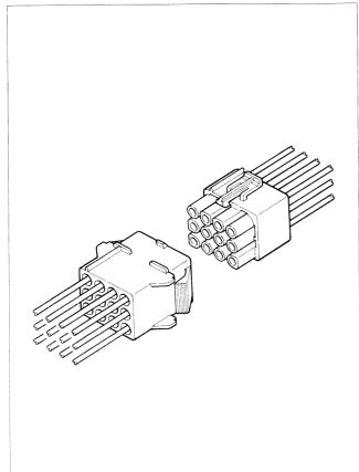
Having the largest power rating in the L connector series, the 600V, 15A LL connector is suited for circuits requiring large electric capacity, such as air conditioner circuits.
