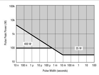
Tentative continuous-pulse allowance at duty is 0.01 %. A load life test with actual equipment is necessary because the curve may be affected by resistance, repetition, duty and derating temperature.
