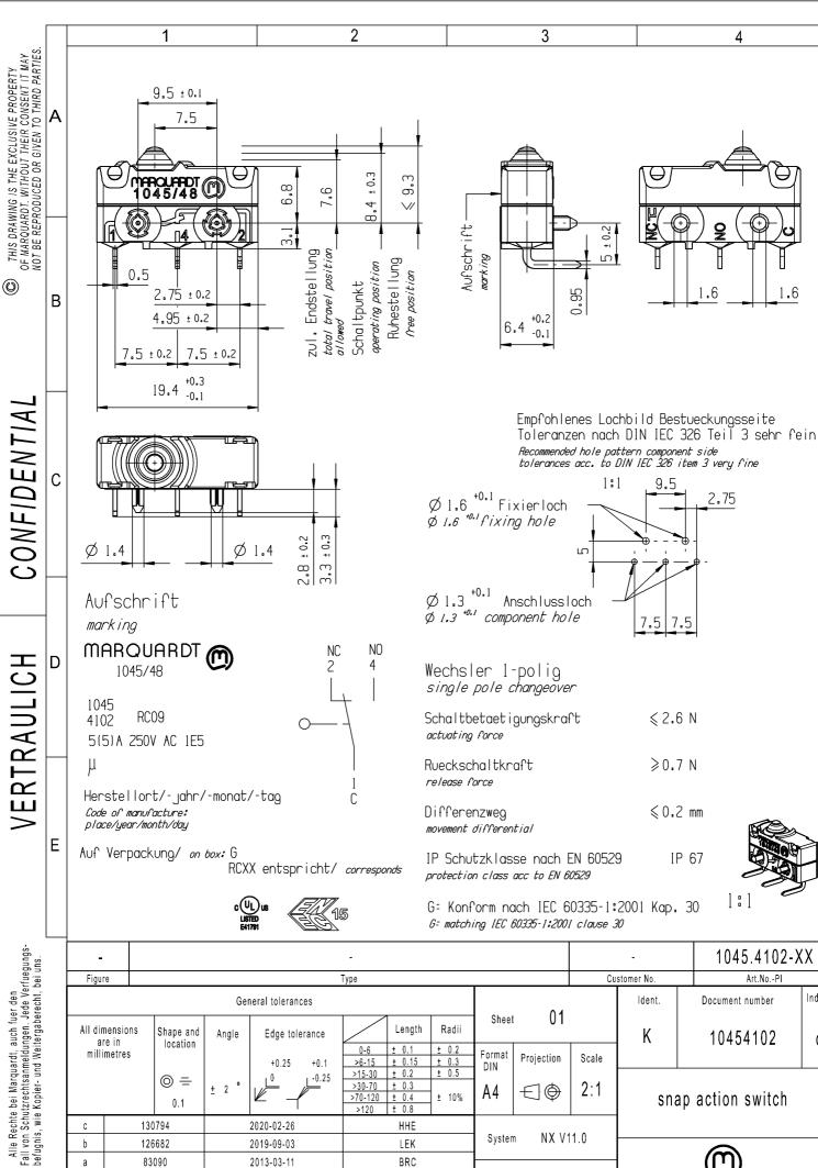
1045.4102-XX Art.No.-PI Document number Index Shape and Edge tolerance Angle K 10454102 C are in location 0-6 ± 0.1 ± 0.2 millimetres Format Projection ± 0.3 ± 0.5 Scale >6-15 >15-30 +0.25 +0.1 ± 0.15 ± 0.2 -0.25 >30-70 ± 0.3 2:1 ± 2  $\bigcirc$ Α4 ± 10% snap action switch 0.1 130794 2020-02-26 HHE NX V11.0 System b 126682 2019-09-03 LEK BRC 83090 2013-03-11 а Replacement of 79865 BRC 2012-09-19 **MARQUARDT** Index MEC-No. Date (YYYY-MM-DD) Edited by
