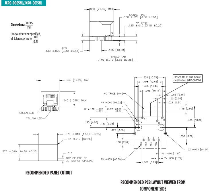
PCB LAYOUT DIMENSIONS REFERENCED TO PIN#1 AND ±.003 UNLESS OTHERWISE SPECIFIED
