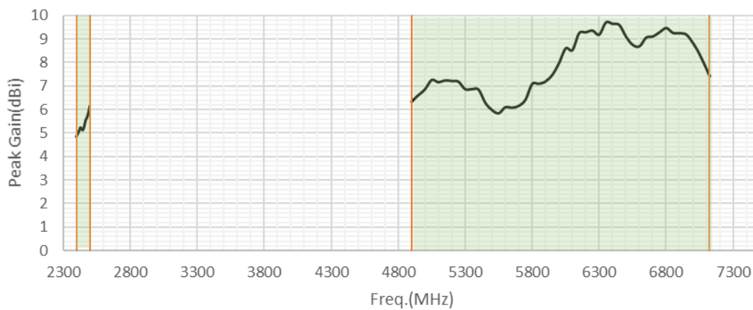
Peak Gain vs Frequency Measured in PSU 20230718
