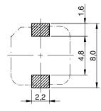
no sensitive traces underneath the component
