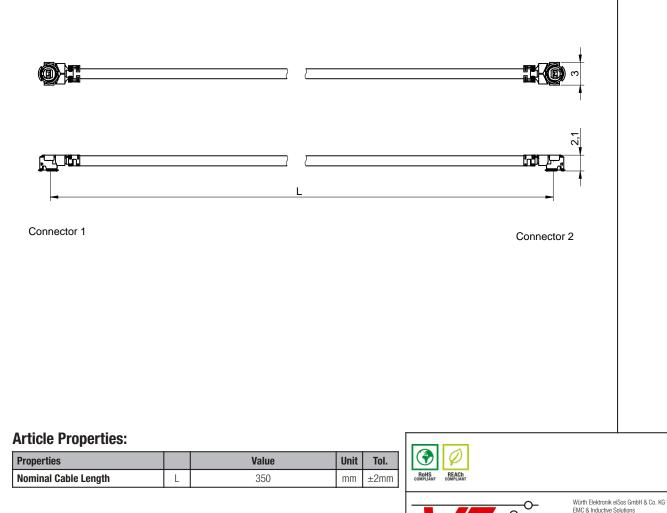
PROJECTION METHOD JTs 001.000 2020-10-27 DIN ISO 2768-1m DESCRIPTION **WR-UMRF UMRF Right Angle Plug** to UMRF Right Angle Plug ORDER CODE 636201070350 SIZE/TYPE STATUS BUSINESS UNIT PAGE Coaxial Cable Dia. 1.32mm Black Jacket eiCan Valid 1/6
