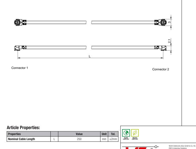
PROJECTION METHOD JTs 001.000 2020-10-27 DIN ISO 2768-1m DESCRIPTION **WR-UMRF UMRF Right Angle Plug** to UMRF Right Angle Plug ORDER CODE 636201070250 SIZE/TYPE STATUS BUSINESS UNIT PAGE Coaxial Cable Dia. 1.32mm Black Jacket eiCan Valid 1/6
