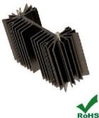
Wakefield-Vette introduces **Universal 678 series**, high performance, low cost and versatile heat sink with screw or clip for all kinds of standard packages. This type of heat sink provides both vertical and horizontal mounting options on PCB to accommodate natural and forced convection cooling method.
