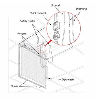
The panel hangers are inserted into the notches on the mounting rail, enabling the panel to hang freely while electrical connections are completed.
