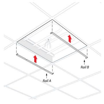
The mounting rails are inserted between the troffer and grid rail on oppositie sides with the anti-rotational tabs pointed inward and notches facing up.
