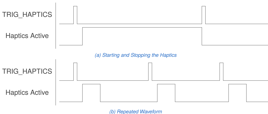
Figure 9.2: Using the TRIG_HAPTICS pin in edge trigger mode. In Figure 9.2a, the second rising edge comes when the haptics is still running. The haptics is stopped. In Figure 9.2b, the waveform finishes before each new rising edge. The rising edges trigger a new waveform.
