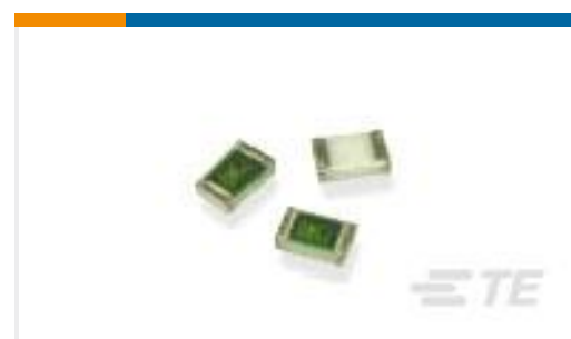
TE Part #5-1879214-5 CPF 0402 1K27 0.1% 25PPM 1K RL
