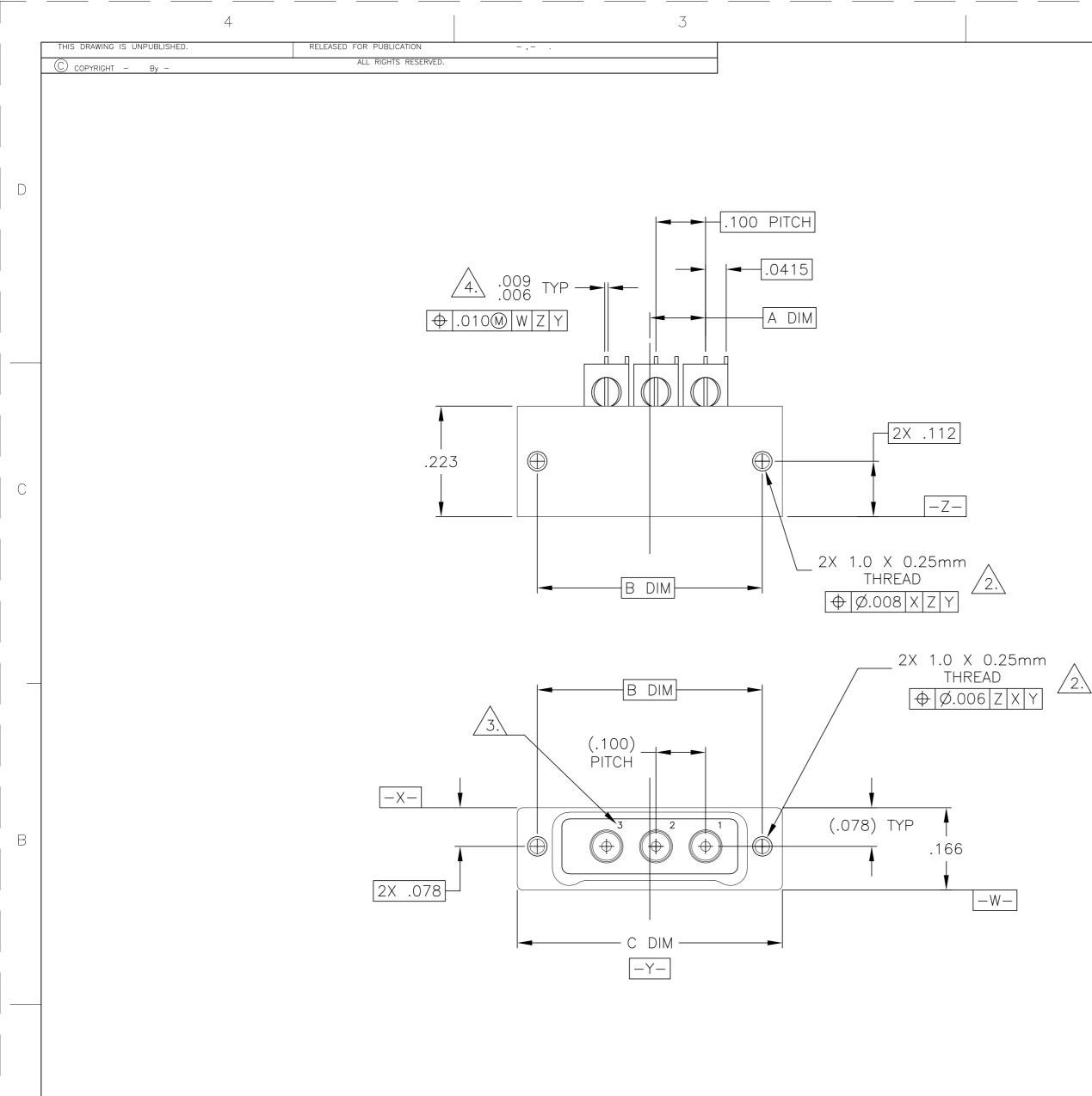
SHELL MATERIAL: 6061-T6 ALUMINUM, ELECTROLESS NICKEL PLATED PER SAE-AMS-C-26074 INSULATOR MATERIAL: LIQUID CRYSTAL POLYMER (LCP) PER MIL-M-24519 OR PER ASTM D 5138
