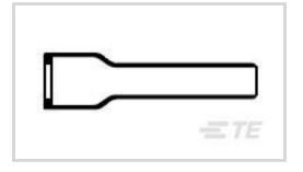
Body Orientation: **Straight** Molded Part Shape Code: **202** Lipped: **Yes**
