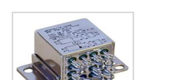
Contact Arrangement: 4 Form C, 4PDT, 4 C/O
